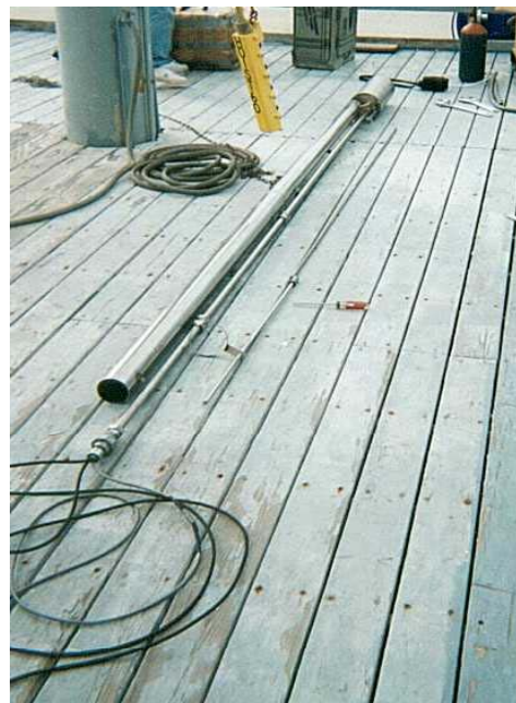
Figure 2. Photograph of the in-tank portion of the LRDP system for a bulk UST with vertical walls.
